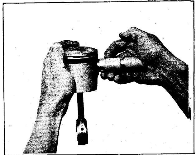
Figure 3C-73. Installing Piston Pin Lock Ring (1979 and Earlier)
