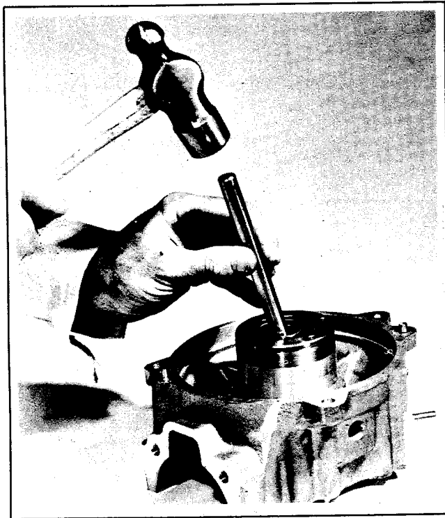
Figure 3E-66. Tapping Circuit Breaker Shaft Bearings from Right Crankcase
